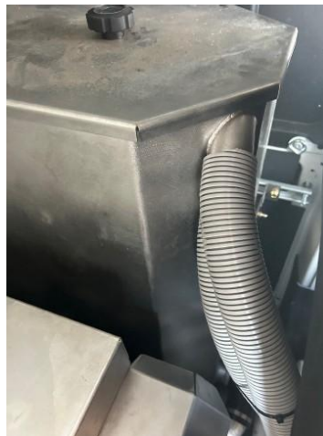
Hoses from the waste tank to the pre-filter box.
